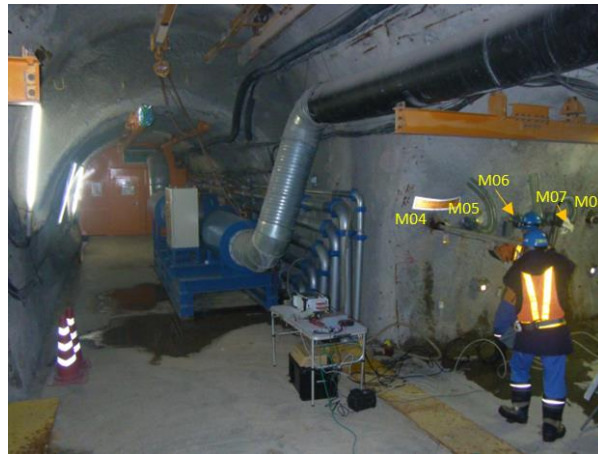
Seismic wave measurement using boreholes.
