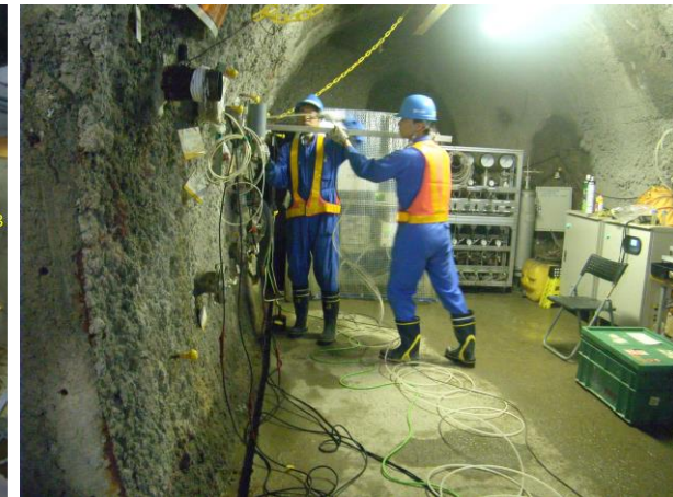
Seismic wave measurement using boreholes.
