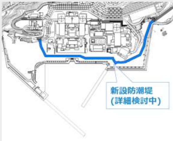
Layout of new seawall
