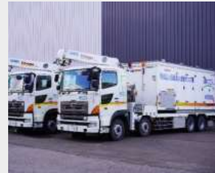
Deployment of two portable large-capacity seawater water pump vehicles
